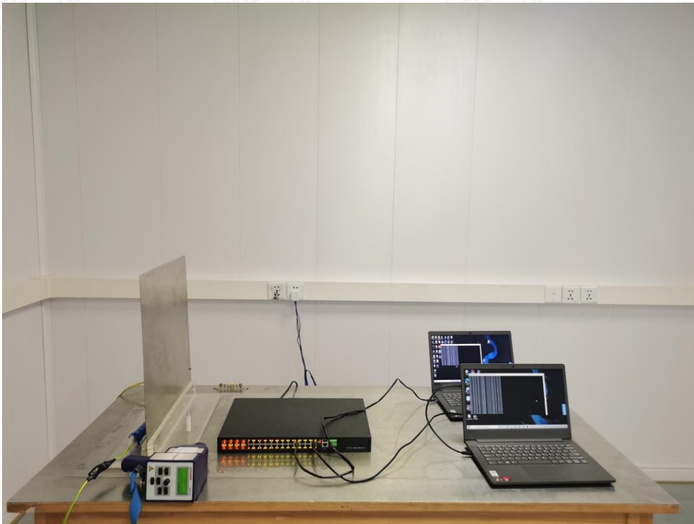
Test Setup Photo of Electrostatic Discharge Test
