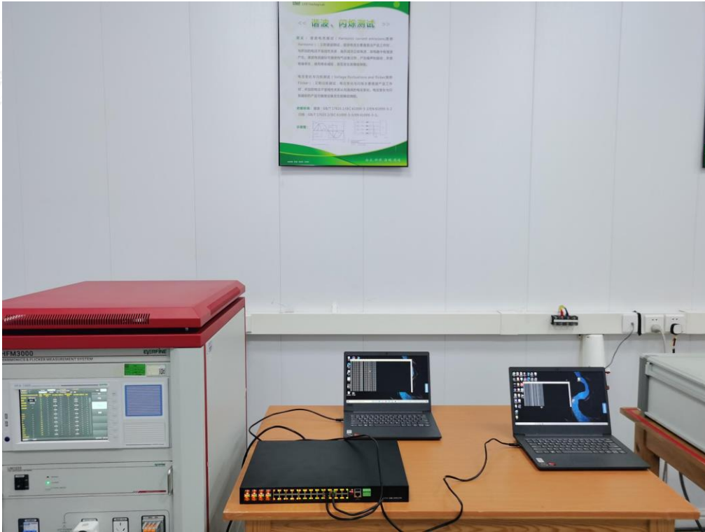
Test Setup Photo of Harmonic & Flicker Measurement
