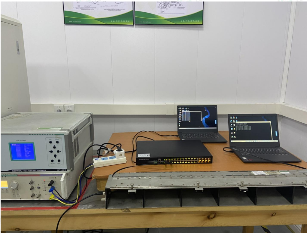
Photo of Signal port Electrical Fast Transient/Burst Test & Surge Immunity Test
