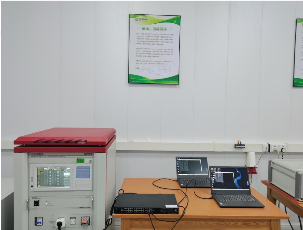
Test Setup Photo of Harmonic & Flicker Measurement
