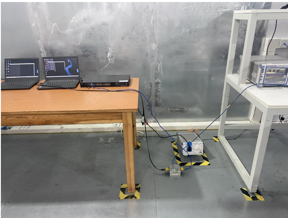
Test Setup Photo of Telecommunication Line Conducted Emission Measurement
